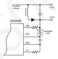
Figure 2: low-side switching supply
