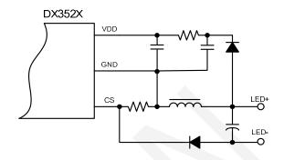
Figure1:Floating ground supply
