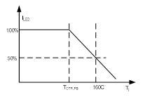
Figure 5: Thermal Foldback Curve
